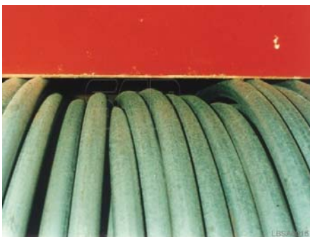
Example of an SGM Magnet handling a loosely wound coil.
