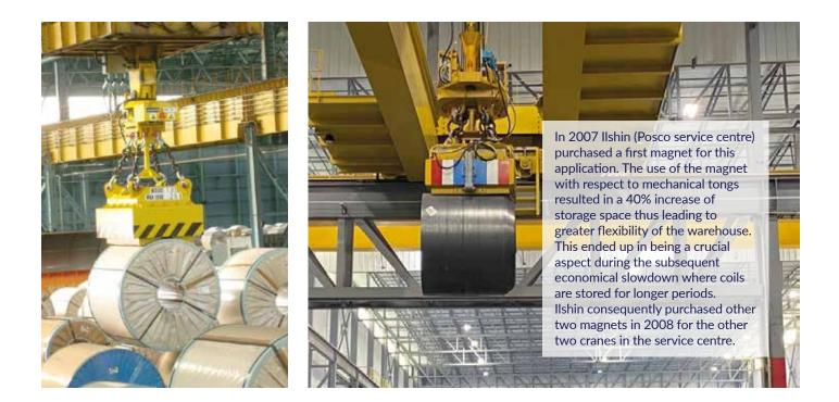
The SGM magnetic system features an exclusive proprietary safety device (CDMD) specifically developed to monitor the two main critical elements that characterise this application:
