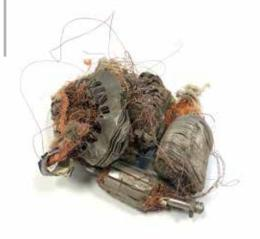
The SGM proprietary Polishing Drum Magnet (PDM) is designed to offer customers the possibility to significantly reduce the quantity of pickers typically used to decrease copper content in the ferrous shred coming off an automobile shredder, which is characterized by the presence of electrical rotors with copper windings (the so-called "meat balls") ending up with the ferrous as a result of their ferrous armature.
