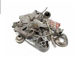
Separation of light metals (aluminum and magnesium) from heavy metals from fines and mid sizes zorba (4mm - 3/16" up to 40mm - 1 1/2")
