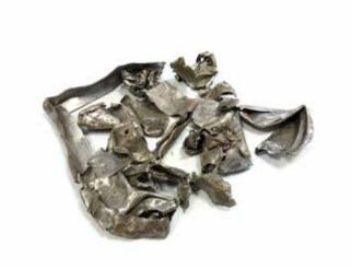
Fines ferrous particles and lightly magnetic material like some austenitic stainless steel pieces
