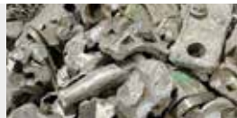
ALUMINUM WITH PIECES OF HEAVY METALS IN THEM OR STILL ATTACHED TO THEM
