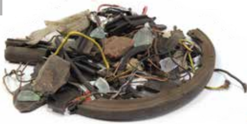
Heavy fraction from SGM Air Classifier going to metal sensor
